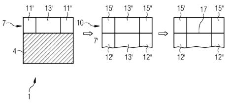
Only in a following step or after having reached a maximum thickness of undensified layers, the inner yet undensified layers 13', 13" are densified in one step
