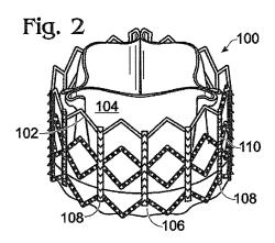
D7 discloses a membrane support (106) with a skirt on the exterior and a thinner ribbon on the interior, for sandwiching a flexible membrane (paragraph [0044]). It also discloses that the membrane support can be affixed to an annular frame (102).
