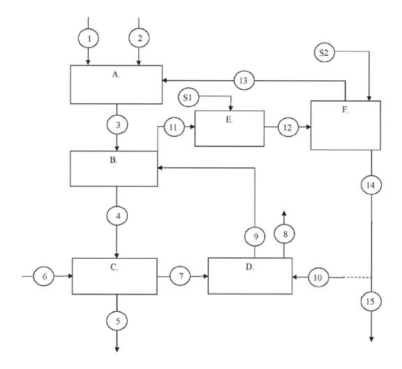
In this process scheme the product formation is on the left side, from A to C. The product (solid urea) is obtained in stream 5.
