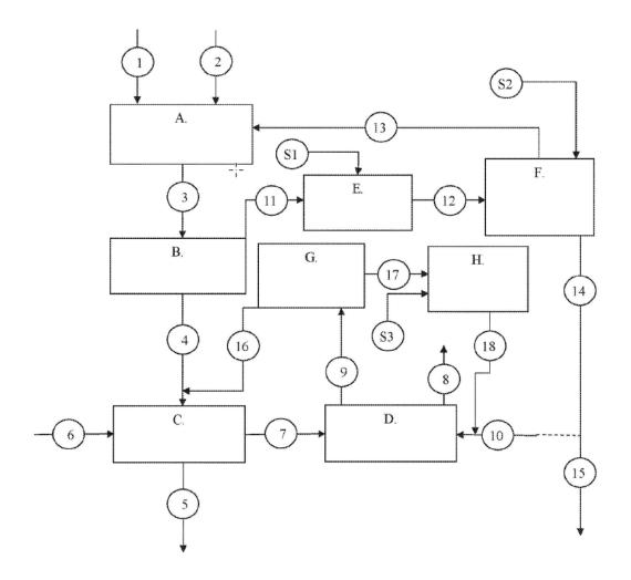
The process contains the additional units G and H, and thus a second evaporation/condensation loop D->G/H->C/D:
