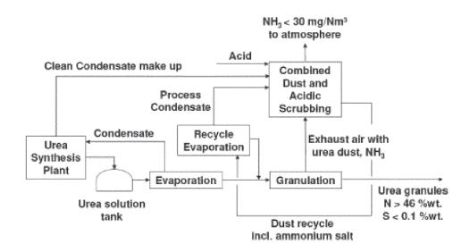
In this figure, the "Evaporation" and "Granulation" units correspond to the evaporation unit (B) and the granulator (C) of the processes depicted above. The "Recycle Evaporation" corresponds to sections G and H of the process of the patent.
