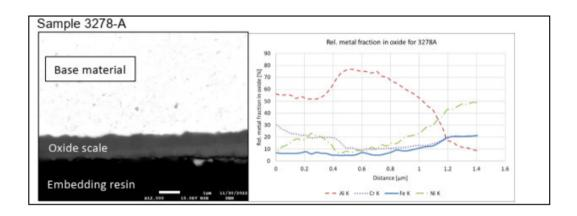
The different grey shadings of the oxide scale in the SEM image and the concentration of Al (dashed line on the top) from 0 to 0.4  $\mu m$  and from 0.4 to 1  $\mu m$  shown by the line scans demonstrate that sample 37 of Dl inherently comprises an aluminium oxide having an Alrich portion on the matrix side and an Al-poor portion on the surface side.
