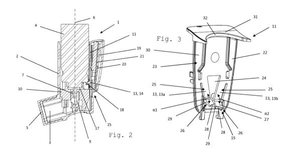
The claimed metered dose inhaler comprises an actuation housing (2), a mechanical dose counter (10), a triggering unit (11) and a processing unit (19).
