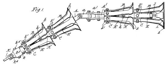
mentioned on page 1, lines 37 to 53 of document D22 link the shaft A of a front unit to the shaft A' of a rear unit. Page 2, lines 75 to 82 of document D22 explains that a socket wrench may be placed into
