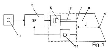
1.2 There are several influences that can impact this signal at the eardrum. First, the hearing instrument could suffer from an "acoustic leakage" after having been inserted into the user's ear canal. Such an acoustic leakage causes the sound pressure at the eardrum to be lower than expected. Secondly, the
