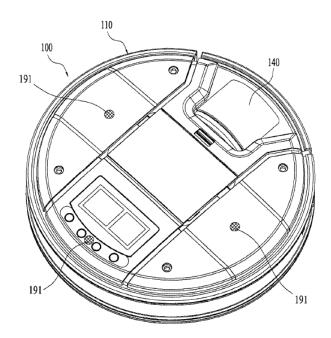
By using sound as a basis for the triangulation, the present invention avoids a typical problem connected with conventional robot cleaners that determine the recharging base's location by means of an infrared (IR) beam where objects can block reception of the IR beam.
