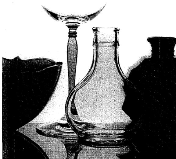
Figure 4. Glass ware demonstrating the still glassy appearance of crystal glass and other types of glasses after being spray coated with hybrid, sol-gel derived layers
