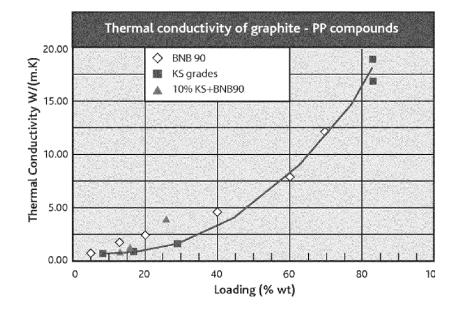
One of the graphites demonstrated is Timrex<sup>®</sup> BNB90 (open diamond on the chart), which is a graphite falling within the scope of the claims, as is seen from paragraph [0046] of the patent in suit and is used in the examples of the patent.
