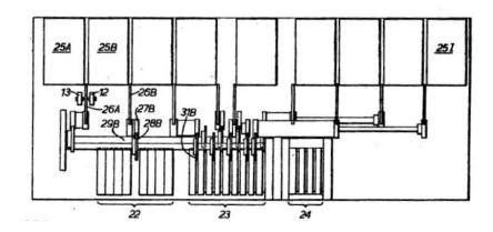
All parties agreed that the nine electric motors 25A to 25I driving the corresponding numbering wheels 23 were not disclosed as brushless DC motors with electronic commutation. In fact, the entire document B53 remains silent as to which type of motors is used for driving the numbering wheels.
