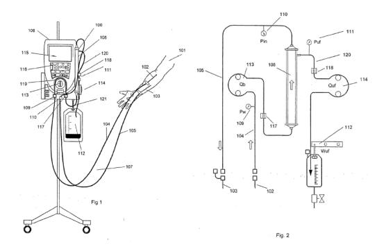
The device comprises an extracorporeal circuit (107), means (needle 102 and blood pump 113) for withdrawing blood from a blood vessel in a patient into the extracorporeal circuit, a blood filter (108) in the circuit for filtering liquid ultrafiltrate from the blood, an ultrafiltrate pump (114) and means (blood pump 113 and needle 103) for infusing the filtered blood back into the patient. The device further comprises a controller which is configured to monitor a
