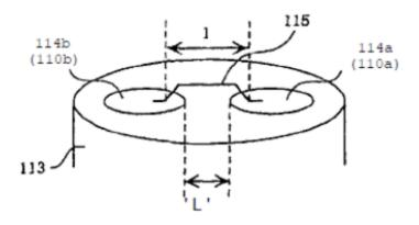
When the welding joints are directly at the edge of the electroconductive bodies (114a, 114b) at the closest point, the two distances 1 and L are clearly the same.
