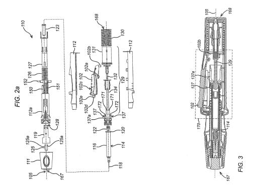
The injection device comprises a housing (112) within which a syringe (114) with a discharge nozzle (118) is received. In use, the syringe is extended in a position in which the discharge nozzle extends from the housing, and its contents are discharged automatically.
