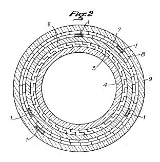
Document D2 teaches the skilled person to provide caisson-shaped wires 1 in the sheathing layers (col. 1,
