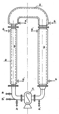
At page 1, lines 25 to 27 of D3, the height to width ratio of the reactor is described as being preferably greater than 5 and the volume of the vertical leg into which the pump discharges as corresponding preferably to about 15% of the total reactor volume.
