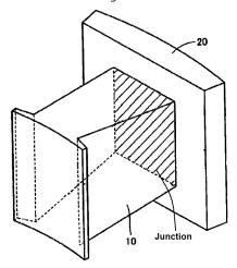
However if that is the case, the last feature of claim 1 is rendered meaningless, and hence unclear, because the cross-sectional area of the junction between the yoke part 20 and each of the plurality of teeth 10 is by definition equal to the area of the cross section of each tooth 10 perpendicular to the radial direction, and cannot be greater than it.
