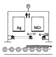
Further, the process run in said chamber lead to an oxidation graded  ${\rm NiCrO}_{\rm x}$  layer deposited on top of a metallic silver layer.
